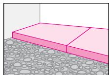
**1. INSTALLING C-300.** Install C-300 over appropriate substrate. Ensure panels are butted together as tight as possible. It's suggested that all joints are taped with approved Owens Corning® JointSealR® tape.
