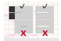
Caution should be taken not to overtighten the screw or bolt that would lead to sidewall deflection into the post. This can be accomplished by adjusting the torque/clutch setting on the drill driver to prevent draw-in.
