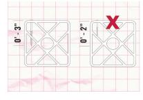
Screws should be at least 3" long to 3.5" long to engage the inner web of the post and prevent cantilever action on the penetration through the sidewall.
