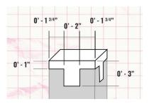
Screwing should be targeted at the outer edge, from 0.25" to 1" from edge, and farther than 1" from end of the post to prevent cracking.
