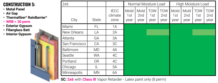
FIGURE 20 – 2x6 wall with WRB = 30 perms and Class III Vapor Retarder.
