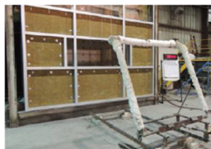
ASTM E2307 intermediate scale, multi-story, test furnace, and the test wall frame used to hold the test wall and perimeter fire containment system.
