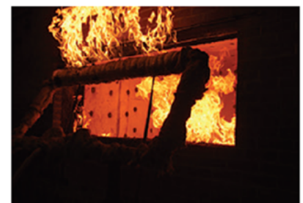
ASTM E2307 room and exterior window burner fire exposure.
