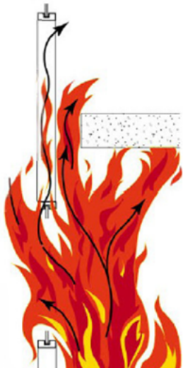
Unprotected Perimeter Joint
