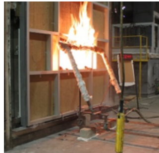
Approximately five minutes into the fire, to simulate vision glass breakage, the window burner is ignited.
