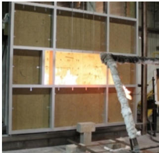
View of the assembly as the fire begins with ignition of the room burner.
