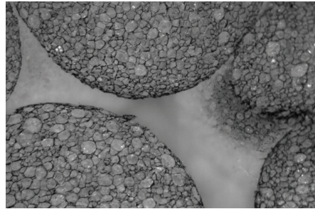
Figure 2: Magnified section of EPS insulation showing gaps between cellular structure.
