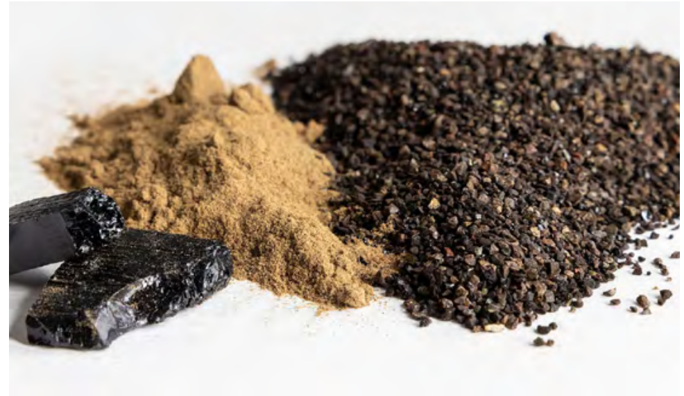
Owens Corning and its partners have successfully deconstructed asphalt shingles into their component parts. Shown above, from left, is asphalt, filler, and granules extracted from waste shingles.
