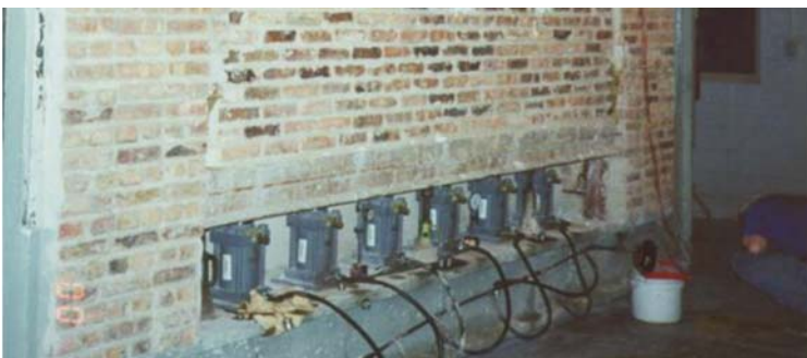
ASTM E119 Test Assembly, Exterior Side
