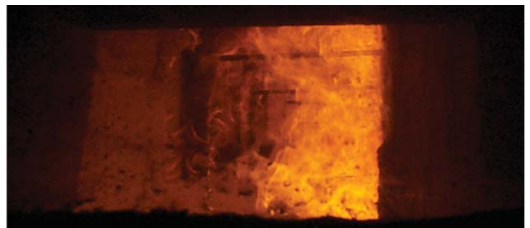
Fire Exposure Inside ASTM E119 Furnace
